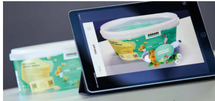
Invisible “Digimarc” barcodes enable IML labels to be separated by type with HolyGrail2.0 technology (photo below). Further product information can be retrieved via AR content (photo above).
