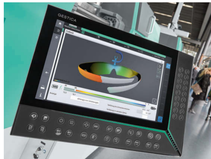
The filling assistant displays the filling degree of the part in relation to the current screw position as a 3D graphic.
