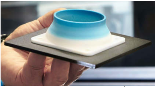
The granulate was dyed in order to produce parts in the typical Festo design colours.
