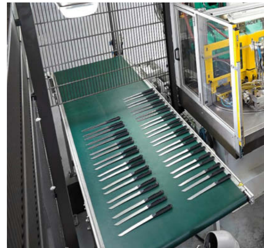
The flexible production cell can overmould around 35 different blade shapes with three different handle sizes.
