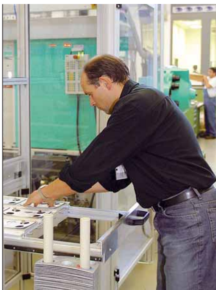
The illuminated moulded part (above) was created by in-mould lamination of special films, which are manually loaded into recesses (below).
