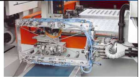
The two-component moulded parts are removed from the mould and palletised in plastic trays by the robotic system.
