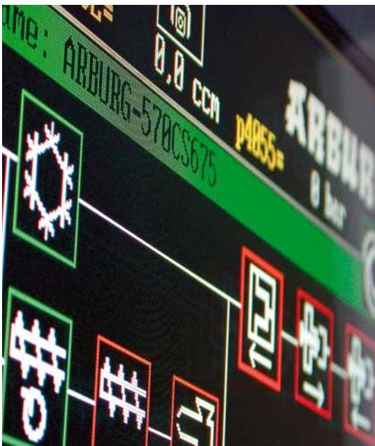
Now and then: Intuitive graphic sequence programming of the SELOGICA (above) and decade switch for controlling machine procedures on the HYDRONICA (right).
