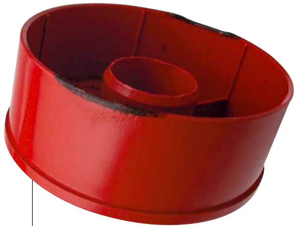
Above: typical moulding defect due to poor ventilation: diesel effect on the flow path end.
